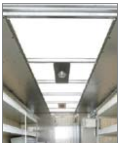
Translucent roof w/30" strip down center aisle or full width
