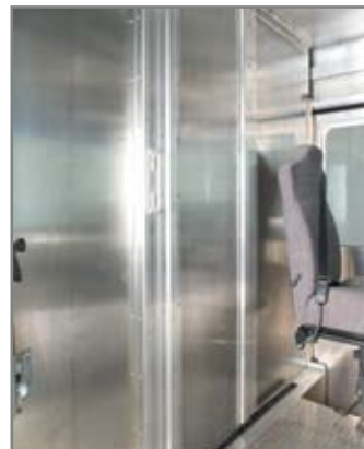
Aluminum bulkhead with center sliding door
