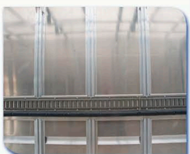
Morgan Olson's patented infinitely adjustable sidewall stiffeners & E-Track provides up and down customization using spring loaded nuts.
