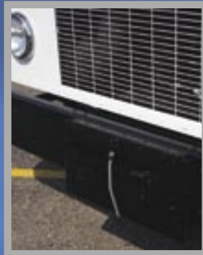
Safety cone holder on front bumper. Solid mount or fold down models available
